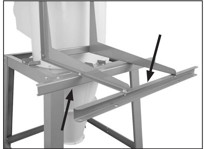
Figure 33. Long brace supports attached.
